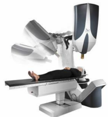
Cyberknife uses linear accelerator mounted on end of
